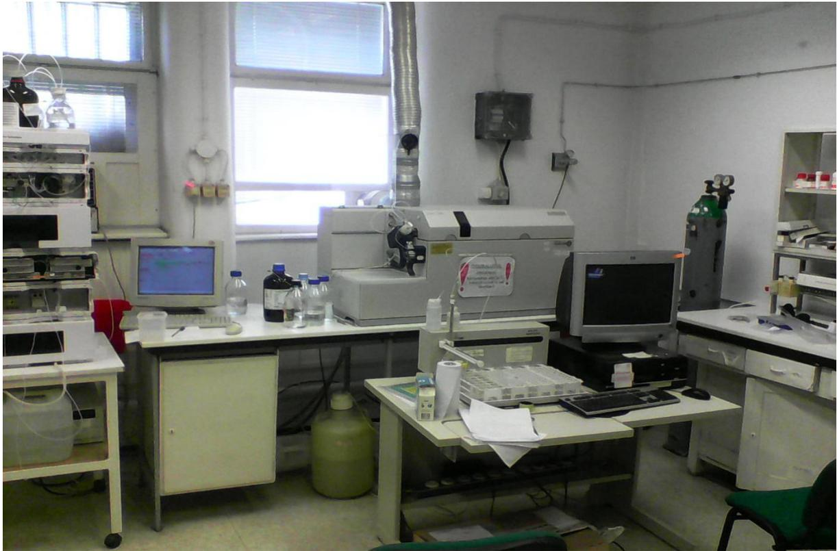
Figure 2: HPLC system coupled by ICP-MS as a detector.
