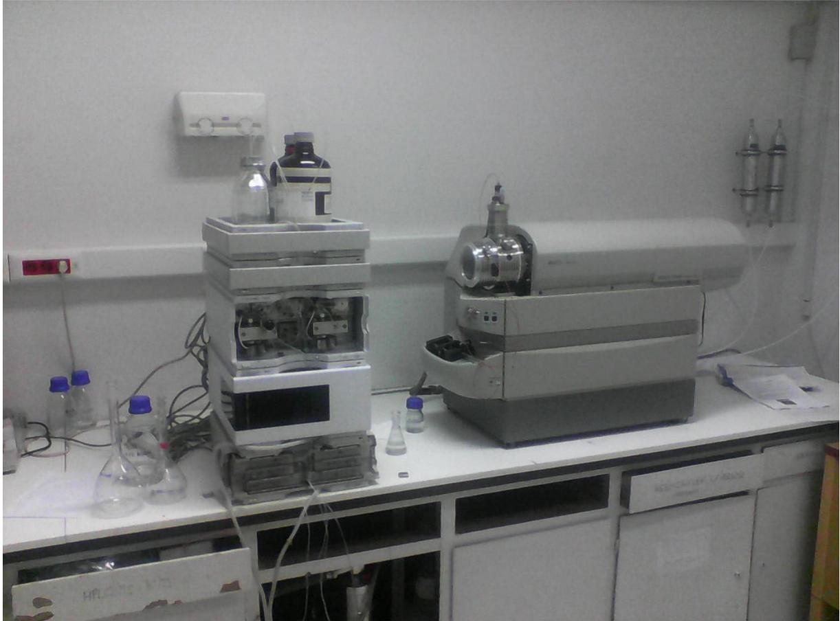
Figure 3: HPLC system coupled by Q-TOF MS as a detector.
